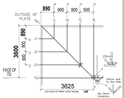
Fix Jack Trusses (J3,J4 Etc) with 1/Triple Grip to Hip Truss and Truncated Girder Truss.
